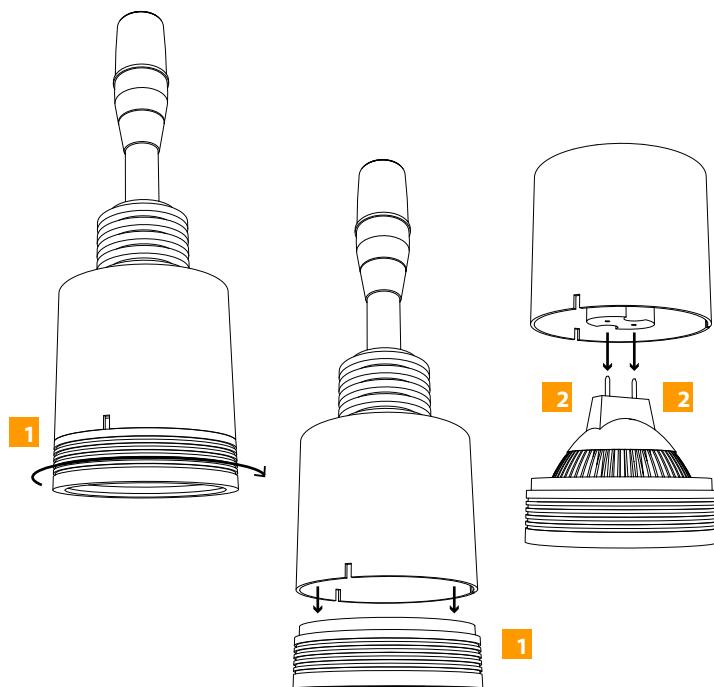
**3** Insert a small hex key, push pin, or paper clip into one hole in the lamp retaining ring and twist counter clockwise to unscrew
